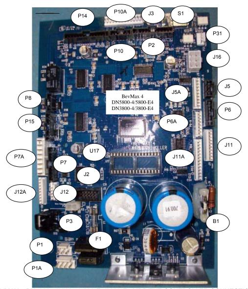
BEVMAX 4 DN5800-4/3800-4/5800-E4/3800-E4 MDB/EXE CONTROLLER CONNECTIONS
