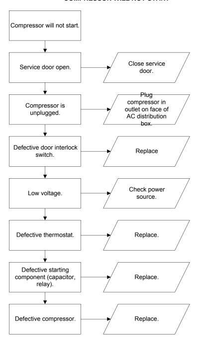
Troubleshooting Tip: Use a short 15 Amp extension cord and plug the compressor directly into the wall outlet. This will bypass the AC distribution box.
